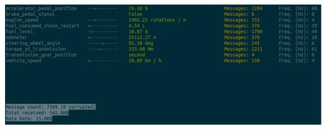
This screenshot shows the dashboard displaying raw CAN messages (the vehicle interface must have CAN passthrough enabled).
